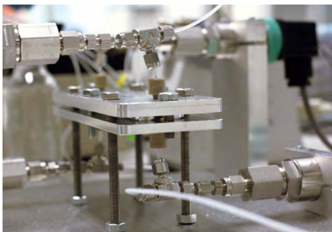
Experimental micro-reactor setup with several inlet and outlet connections.
